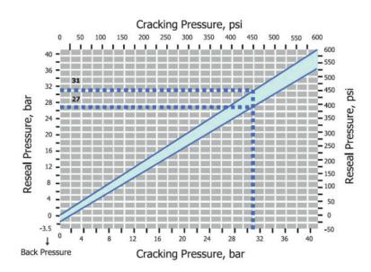
Example shown : For a valve set to crack at 31 bar (450 psig), the minimum reseal pressure would be 27 bar (390psig).
